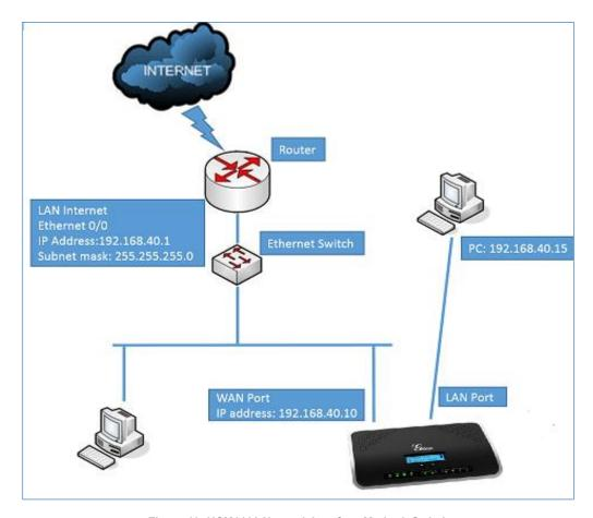
Figure 13: UCM6102 Network Interface Method: Switch
