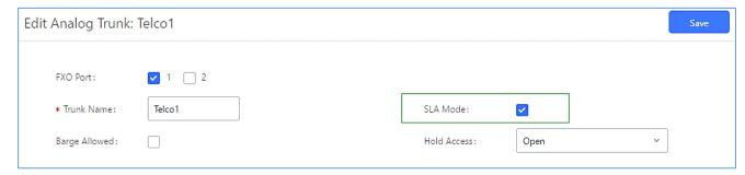
Figure 103: Enable SLA Mode for Analog Trunk
