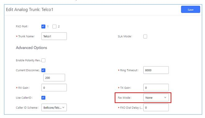
Figure 169: Configure Analog Trunk without Fax Detection
