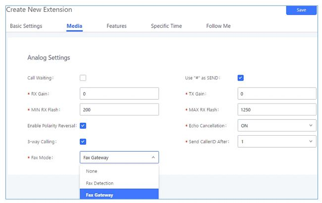
Figure 171: Configure Extension for Fax Machine: Analog Settings
