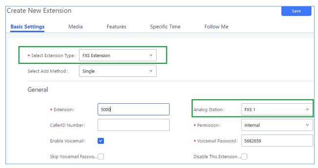
Figure 170: Configure Extension for Fax Machine: FXS Extension
